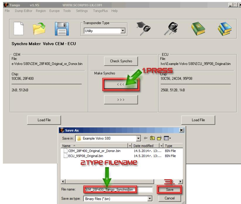
After the new file is generated it is advised to check the synchronization before applying it to the module. Following the example, Press "Load File" under CEM section within the software and select the newly generated by Tango file, which was created in the step above:
