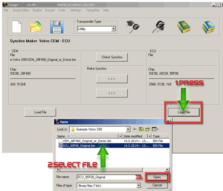
If you press the **Check Synchro** button now, it will display the following error, because at this point the files of the ECU and CEM **are not synchronized**. **NB:** If the files are taken from a working car the error will not appear and will write "SUCCESS" instead.
