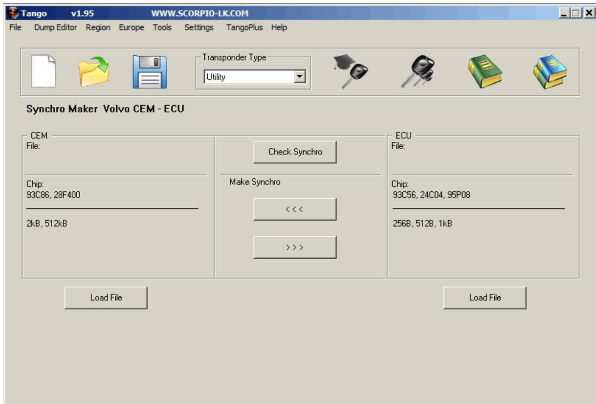
The Synchronization of the modules begins with loading their dump files in Tango software, in the example used in this document the sync between CEM with 28F400 and ECU with 95P08 will be displayed. **It doesn't matter which file is loaded first.**
